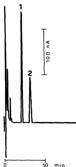
Fig. 6. Analytical profile obtained on applying method D to a plasma containing (1) Co Q 9 (I.S.), 2.50 mg/l, and (2) Co Q 10 , 0.92 mg/l. Column-switching precolumn, C 18 , 40–60 \mu m (20 mm \times 2 mm I.D.). Analytical column, mobile phase and detector as in Fig. 5. Integrator attenuation, 512; chart speed, 5 mm/min.
